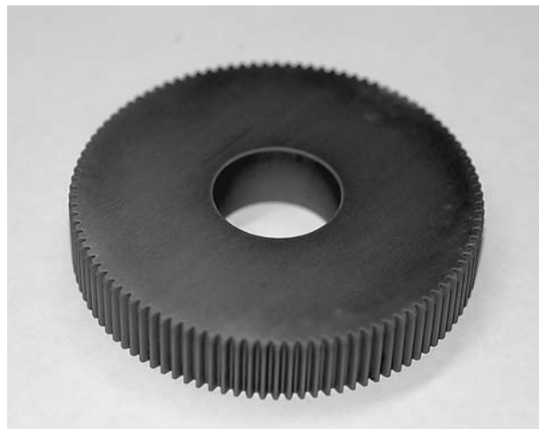
Fig. 3 Appearance of electrical discharge machined SAN-3 ceramics.
